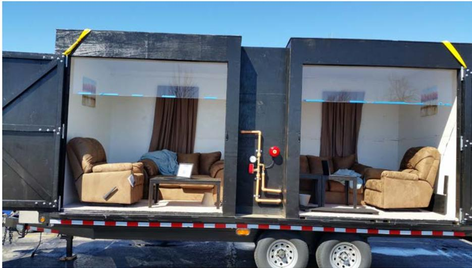
NFSA WI received the second mobile side by side trailer for fire sprinkler demonstrations that show how fast fire grows and the effectiveness of fire sprinklers on protecting lives and property. The first side by side was delivered Fall of 2017 and has been in use in the Green Bay area since. This demo unit allows for ease of transportation to sites and return for reset. It has increased the number of side by side demonstrations when in use across the U.S.
